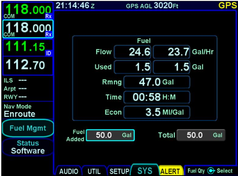
If the fuel flow system is not capable of reporting the amount of fuel remaining (i.e. does not have a totalizer), then the IFD will present two controls allowing the fuel quantity to be manually adjusted.
