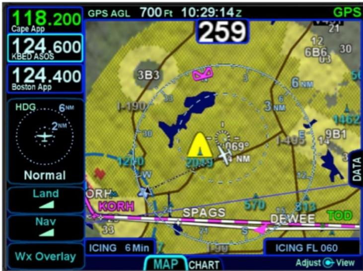
Terrain Awareness coloring can be triggered by terrain within a 10nm radius of the aircraft and is displayed as follows, depending upon the installation:
