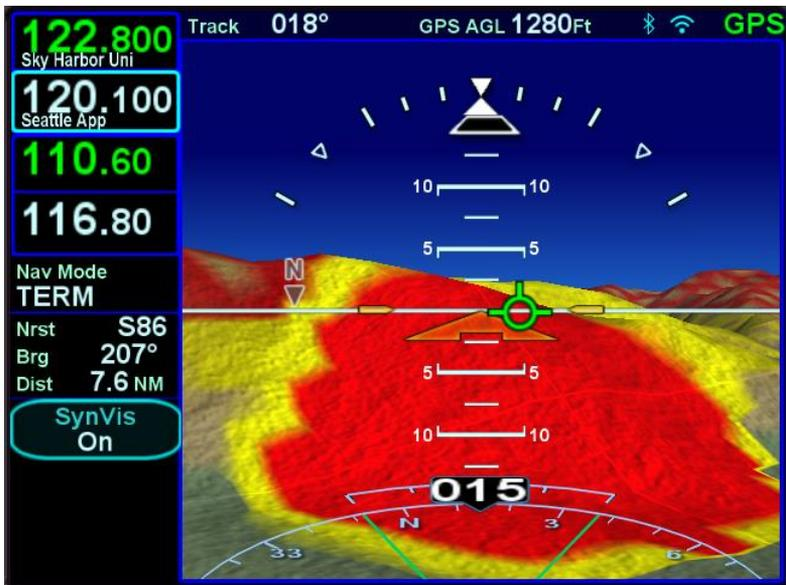
Either terrain or obstacles can trigger FLTA alerts and they are distinguished via the CAS messaging and aural alerting. The difference between FLTA warnings and cautions is exclusively based on distance-to-go to projected impact points or reduced clearance areas.
