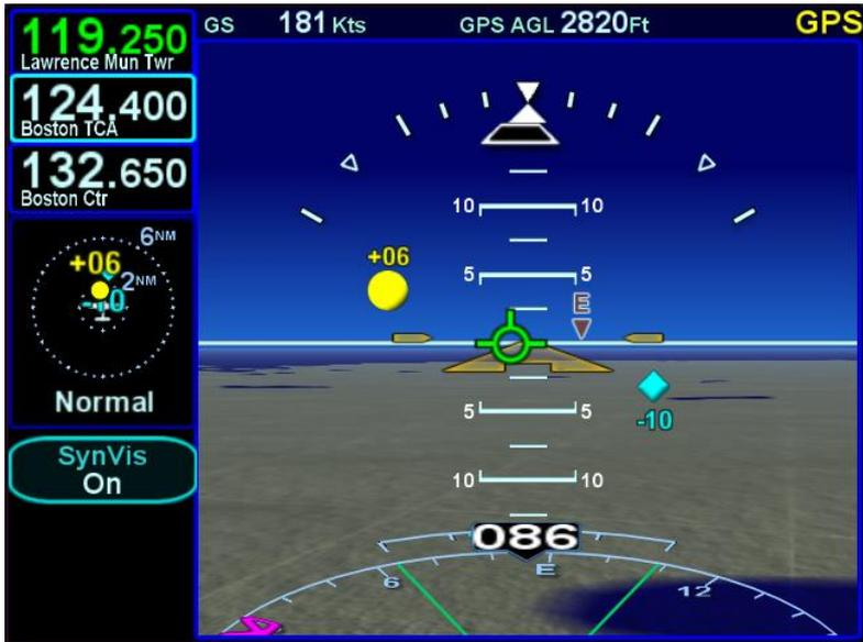
The TVV will grow in size when it is behind the deviation indicators or heading digital readout bubbles in order to stay viewable.
