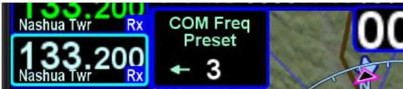
If the com preset page is displayed at the time the cockpit control is activated, a small arrow will indicate which preset is tuned.
