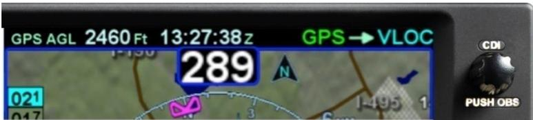
The IFD510 nav source button is similar to the nav source knob, except that it toggles only between GPS based navigation to the flight plan and an OBS course to the active waypoint.
