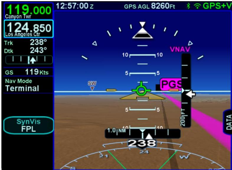
Vertical deviations will continue to be provided along the descent until the target altitude has been reached. During descent, if the aircraft deviates from the intended flight path by more than 2nm or if the aircraft course deviates by more than 45 degrees from the desired track, enroute VNAV deviations will be flagged until the aircraft resumes flight along the flight plan.
