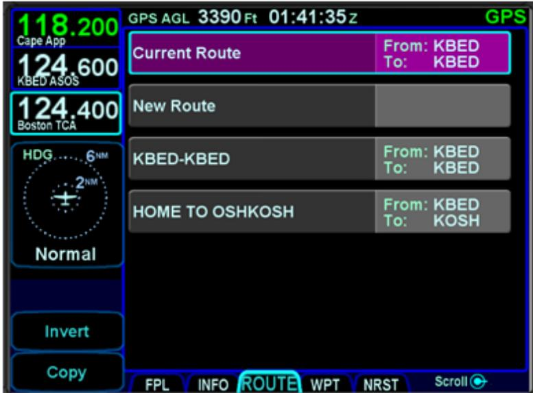
As indicated in the above image, each stored route is represented by a single row with the route name on the left and the "from" and "to" points identified on the right side of the row. Additionally, there are two special purpose rows shown at the top of the list.
