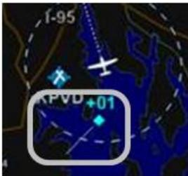
Since TIS-A traffic data is re-radiated data from FAA ground stations, there are a few additional possible states of the data beyond normal operating state. The non-normal TIS-A status states will be displayed in the traffic thumbnail and as CAS messages and include:
