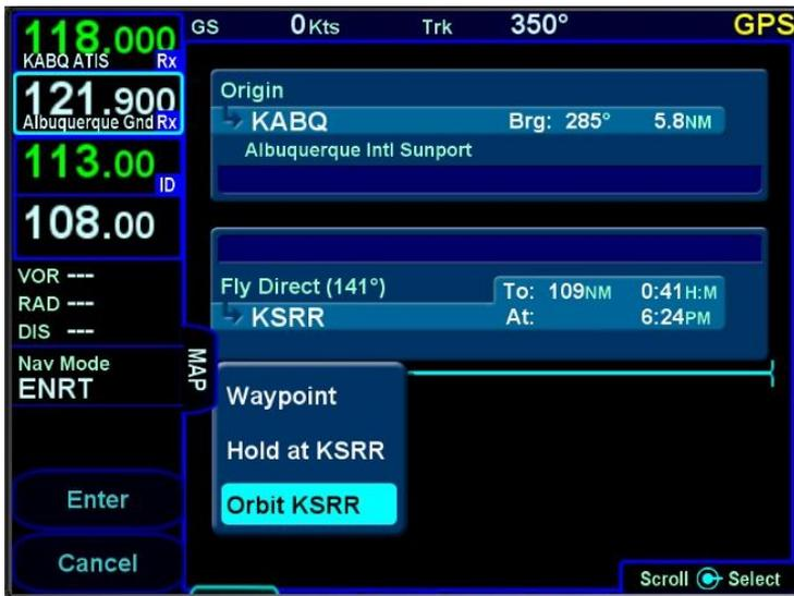
The orbit radius can range from 0.5nm to 100nm. The FMS will not actually fly to the orbit fix and instead, will fly to the point where the leg to the fix intercepts the orbit.
