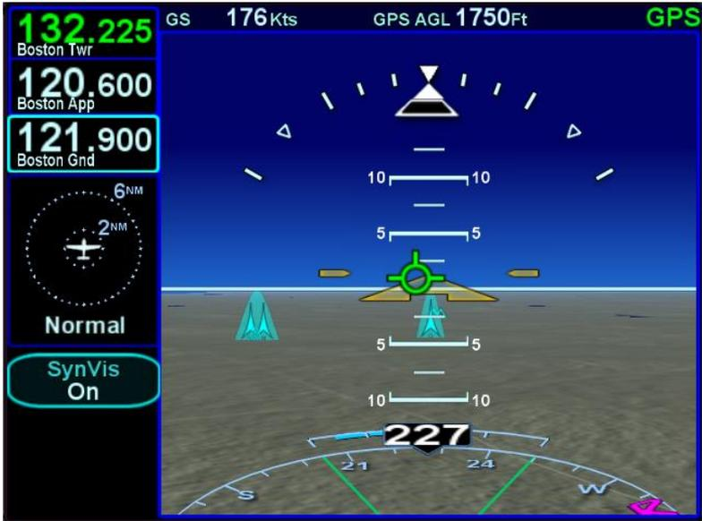
Obstacles inside a 3nm radius of the aircraft position and whose top is between 100' below aircraft altitude and 1000' below aircraft altitude will generate a yellow threat bubble over the obstacle on the SynVis scene and the map pages.
