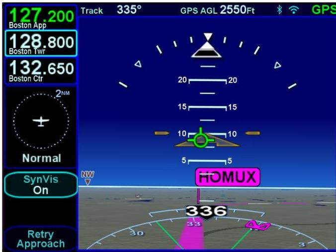
Deviations are indicated by both the SynVis scene depiction and the horizontal and vertical deviation indicators. In the image below, the airplane is displaced to the right of final and is well above glideslope. A pegged deviation indicator is displayed in yellow.
