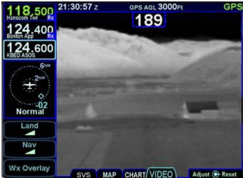
The video image can be pinch zoomed using two-finger touch pinching gestures on the glass and finger panned. The pinch zooming range is 1x to 5x magnification.
