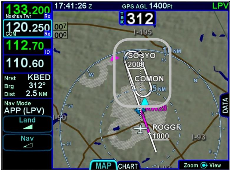
When executing the missed approach, apply go-around power, establish a climb attitude, reconfigure the aircraft as necessary, ensure the aircraft is trimmed properly, and consider using the autopilot to smoothly execute the assigned or published missed approach.
