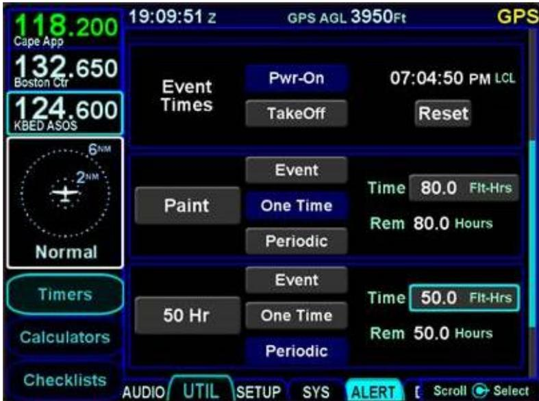
Acknowledging the alert when a custom timer has expired (via touch or pressing the CLR button) will clear the alert message, but will not delete the timer.
