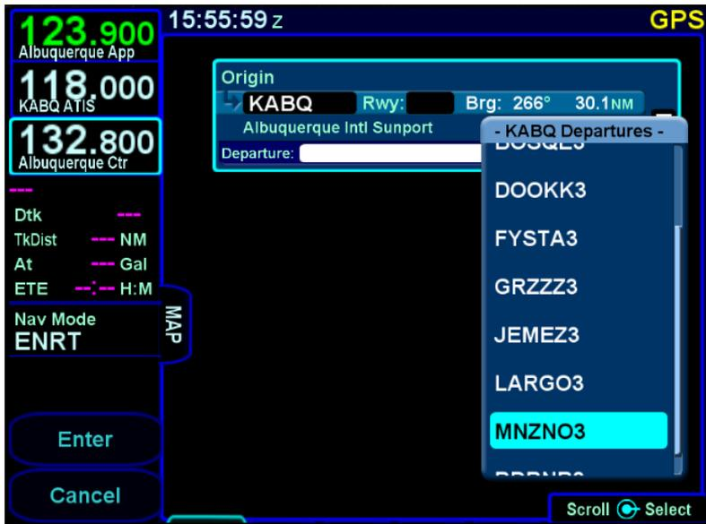
When a departure is selected from the initial dropdown, a sequence of dropdowns may be presented to allow the selection of an enroute transition and a runway transition. The structure of the departure and the presence of a selected runway will impact whether a specific dropdown is presented.
