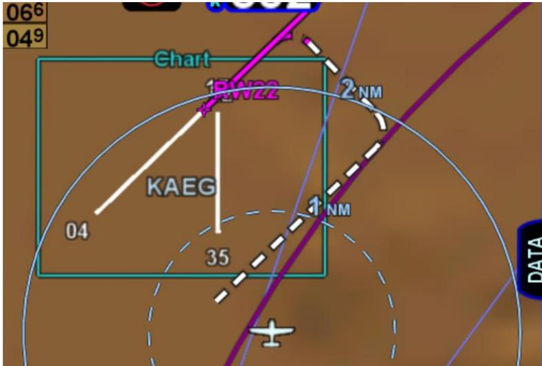
When flying a visual approach, lateral deviations are provided to the final approach course. Advisory vertical deviations are also provided once the aircraft track is at most 90 degrees to the final approach course. Therefore, on a downwind entry the VDI will remain flagged until the aircraft completes the turn to base.
