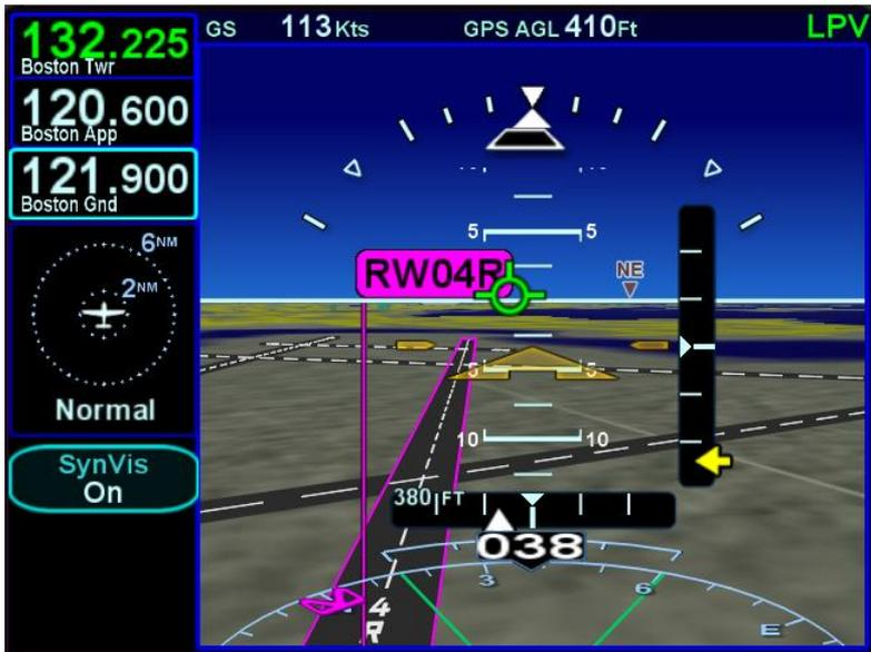
The Setup Page provides a means to control whether cardinal heading marks are shown along the horizon line.
