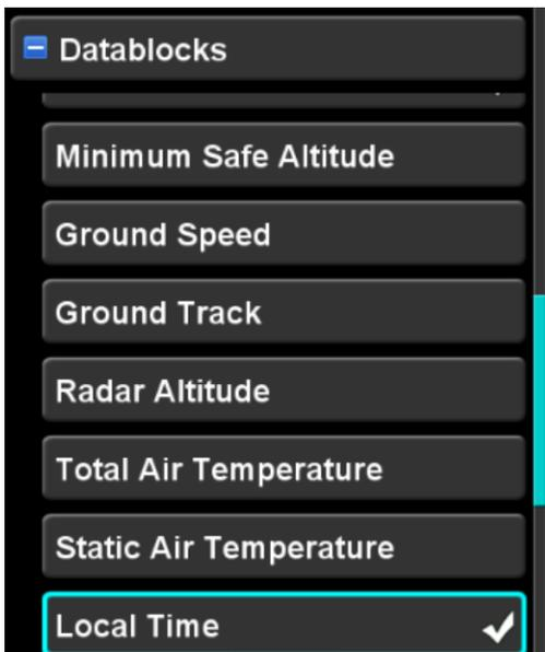
Once the datablocks category is expanded, the operation of the right knob is slightly different than the normal Setup Page operation. The outer knob selects the datablock “slot” to be affected. The inner knob selects the datablock that is to be displayed in the selected slot. The selected slot is shown with a blue background (except for the VLOC radio block). The selected datablock is shown with the typical cyan cursor surrounding the item.
