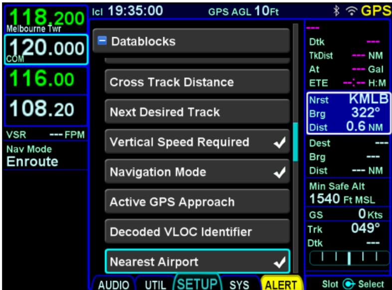
In order to change the datablock selected in a given slot, first turn the outer knob or touch to move the cursor to the desired slot. Then, use the inner knob or touch to select the datablock item to be displayed. Then, press the knob button or touch the datablock again to place it into the selected slot.
