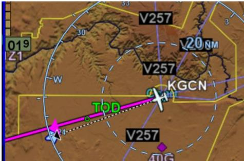
When a target vertical speed is specified, the IFD will compute the TOD point using current groundspeed and the desired descent rate. However, when the aircraft reaches the TOD point and enroute VNAV is allowed, the IFD will compute the angle required to reach the desired altitude, then commence with enroute VNAV using that angle.
