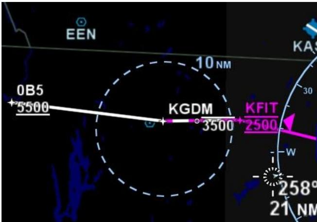
The altitude constraint depiction will also appear at the proper geographic position. For example, if an altitude constraint were defined to be 5nm prior to a waypoint like it is for KGDM in the image above, the graphical representation of the altitude constraint on the map will be positioned 5nm prior to the waypoint, instead of at the actual waypoint.
