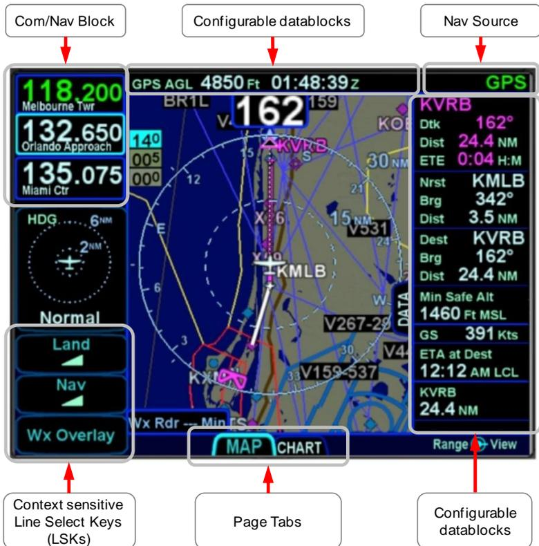
Each page has a number of associated tabs. To select a tab using the page key, press the left or right side of the key to move left or right, respectively, among the tabs until the desired tab is selected. To select a tab using the touchscreen, just touch the
