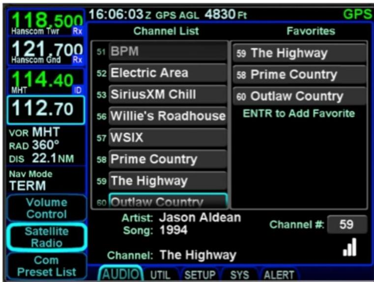
The page is divided into three parts. The left side of the page is a full channel list of all available satellite radio channels. The right side of the page is a numbered list titled “Favorites” and represents the satellite radio channels that have been programmed into a preset list for faster access. The bottom of the page contains a datablock indicating the artist, song, channel name and number, audio signal strength and a Quick Go To link to enter in a desired satellite audio channel.
