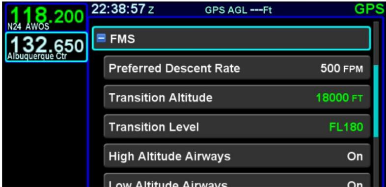
The transition altitude advisory CAS message is displayed when the aircraft climbs to within an altitude 250 feet below the transition altitude. Once issued, the alert will not be eligible to be issued again unless the aircraft has descended more than 500 feet below the transition altitude.
