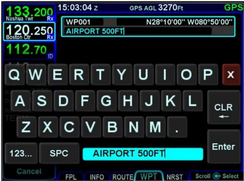
When used in a flight plan, the user-defined airport will display as an airfield with no known runway orientation.
