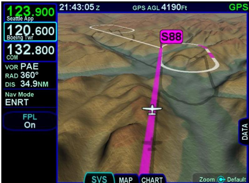
Any traffic in the scene will cast a shadow on the ground to help with judging distance and relative closure rate.
