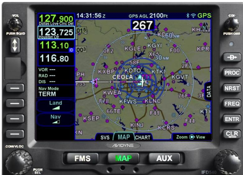
Supplemental IFD functions include a moving-map, flight management system (FMS), electronic charts, checklists, and a number of timer and calculator types of utilities. Optional IFD functions include control and display of remote transponders,
