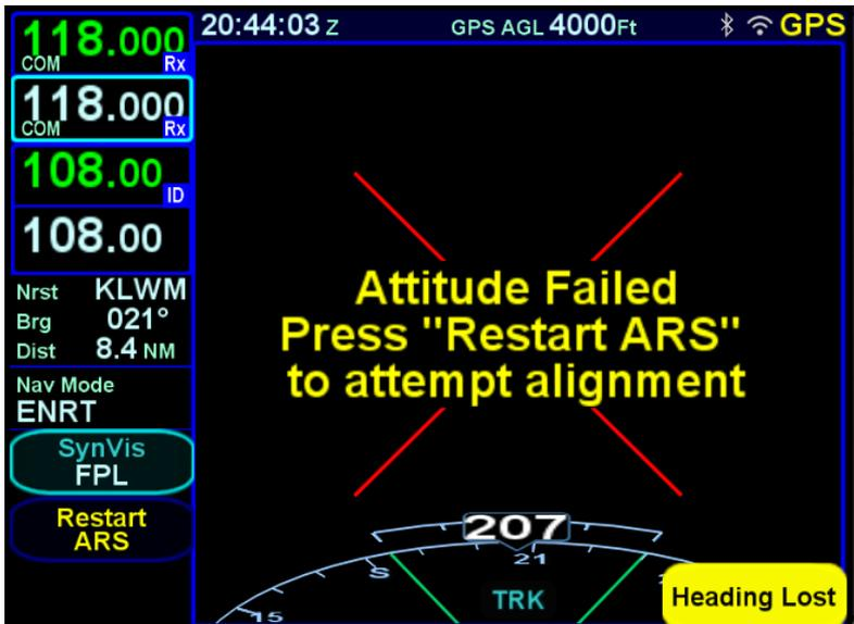
If the ARS data (mark pitch, roll and heading) becomes invalid, the ARS page will display a red "X". Once the aircraft has returned to straight and level flight, press the "Restart ARS" button or soft key and maintain straight and level flight for at least 30 seconds.
