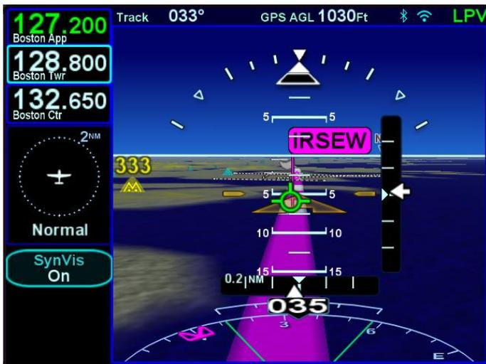
The active runway in the FMS flight plan is highlighted with a magenta outline drawing the airfield identifier flag is “planted” at the runway threshold, if known, or airport reference point if not.
