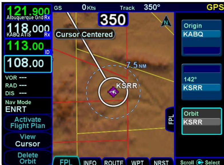
The function is activated on the Setup Page by setting the "Patterns" field to "On".
