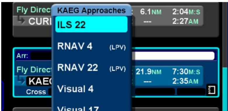
Once a visual approach has been selected, the familiar transition dropdown will appear. The dropdown contains selections for a straight-in approach and for base and downwind pattern entries using both left and right turns, as illustrated below.
