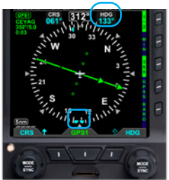
Figure 2-5 HDG field updated and inactive
