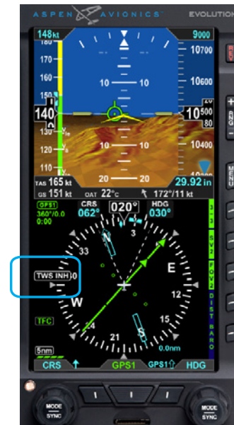
Figure 4-149 TWS Inhibit Display
