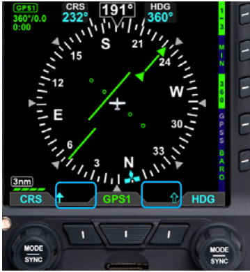
Figure 4-75 Bearing Pointers OFF
