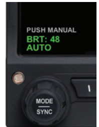
Figure 3-6 Display Brightness in AUTO Mode
