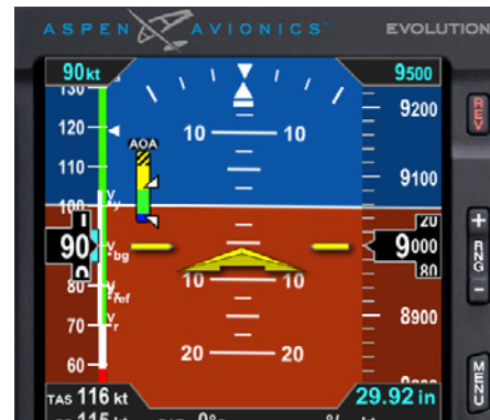
Figure 4-113 Angle of Attack (AOA) Display
