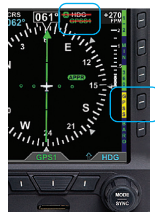
Figure 4-109 GPSS Automatically Disabled — Wings Level Mode
