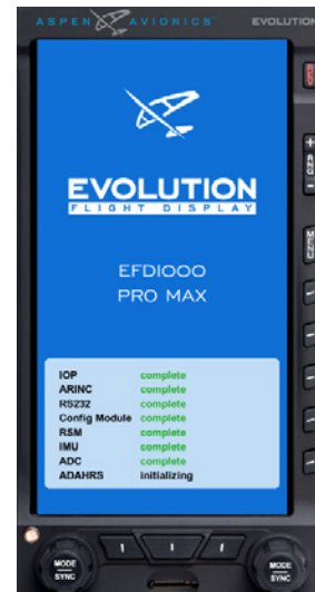
Figure 3-2 EFD1000 Pro MAX PFD Startup
