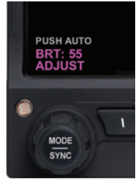
Figure 3-5 Display Brightness in ADJUST Mode
