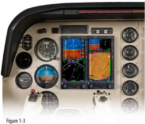
Figure 1-3 Dual Display System: PFD & MFD
