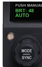
Figure 2-17 Display Brightness in BRT AUTO Mode
