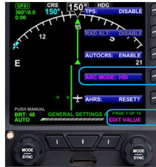
Figure 4-43 Changing the ARC Compass MODE
