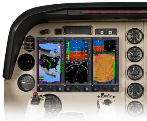
Figure 1-4 Trio Display System: PFD & Dual MFDs
