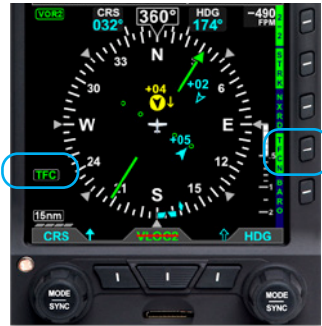
Figure 4-100 Traffic Overlay Enabled
