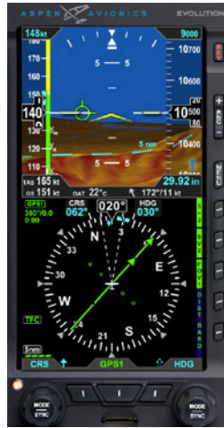
Figure 4-135 FOV1 Narrow Field of View
