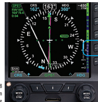
Figure 4-108 GPSS Disabled and Autopilot in HDG Mode
