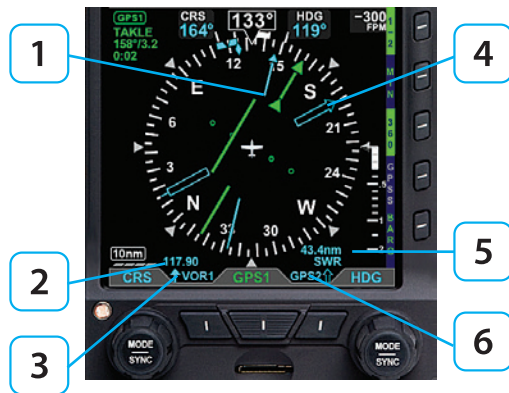
Figure 4-74 Bearing Pointer Description
