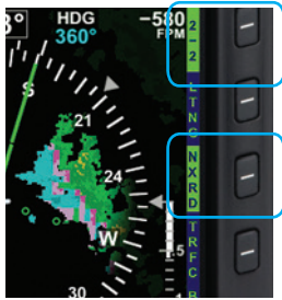
Figure 4-97 Data Link Weather Enabled
