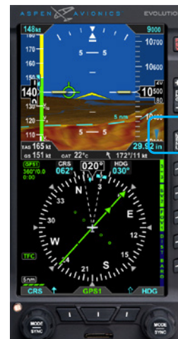
Figure 4-128 Narrow Field of View (FOV1)
