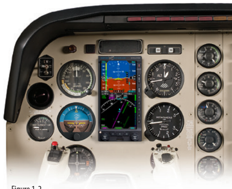
Figure 1-2 Single Display EFD1000 Pro MAX PFD System
