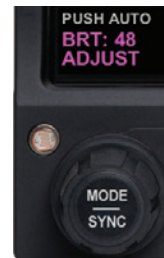
Figure 2-18 Display Brightness in BRT ADJUST Mode
