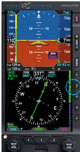
Figure 4-27 MIN Hot Key – Selected Minimums
