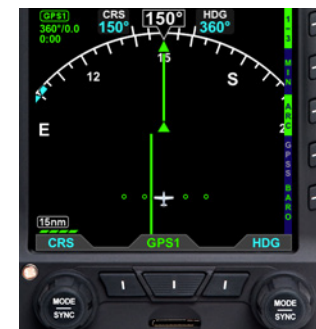
Figure 4-40 ARC HSI Compass Mode
