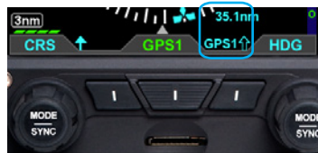
Figure 4-79 Double-Line Bearing Pointer and Button
