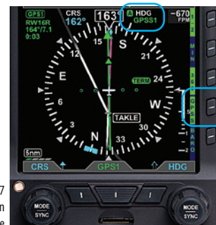
Figure 4-107 GPSS Enabled with Autopilot in HDG Mode
