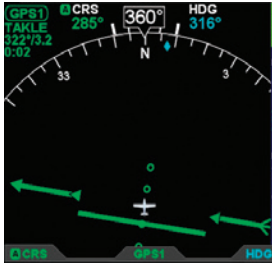
Figure 4-46 Reduced Length Course Pointer, ARC HSI Compass Mode
