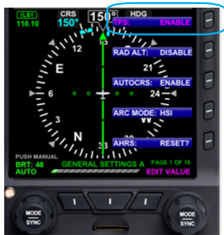
Figure 4-16 Editing Airspeed Tape Display
