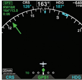
Figure 4-47 Stub Course Arrowhead, ARC CDI Compass Mode
