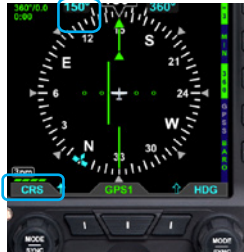
Figure 4-73 CRS Field Enabled for Editing
