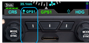
Figure 4-78 Single-Line Bearing Pointer and Button
