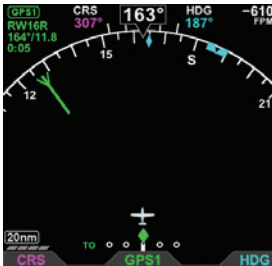
Figure 4-48 Stub Course Tail, ARC CDI Compass Mode
