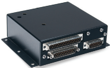
Figure 1-8 Analog Converter Unit (ACU)
