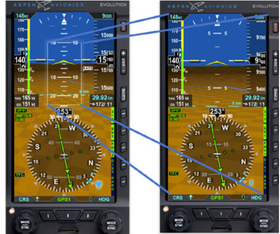
Figure 4-138 FOV1 Narrow Field of View
