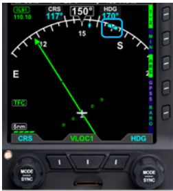
Figure 4-81 Heading Bug and Selected Heading Field
