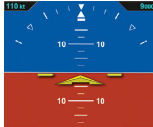
Figure 4-17 Airspeed Tape Disabled
