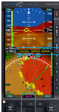
Figure 4-148 Terrain Alert, Synthetic Vision VIEW
