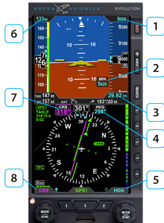
Figure 2-3 Left and Right Knobs and Corresponding Fields
