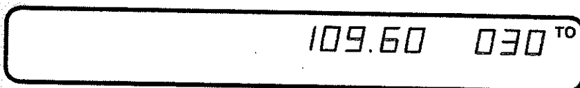
VOR MODE: ACTIVE "BEARING TO" FUNCTION DISPLAY
