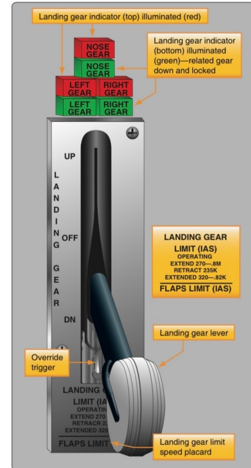
Figure 11-10. Typical landing gear switch with three light indicator.
